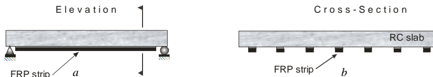
Fig. 7. – FRP strengthening of one-way simply supported plate: a – elevation; b – cross section
