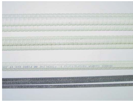
Fig. 1. – Types of FRP composite reinforcing bars for concrete elements
