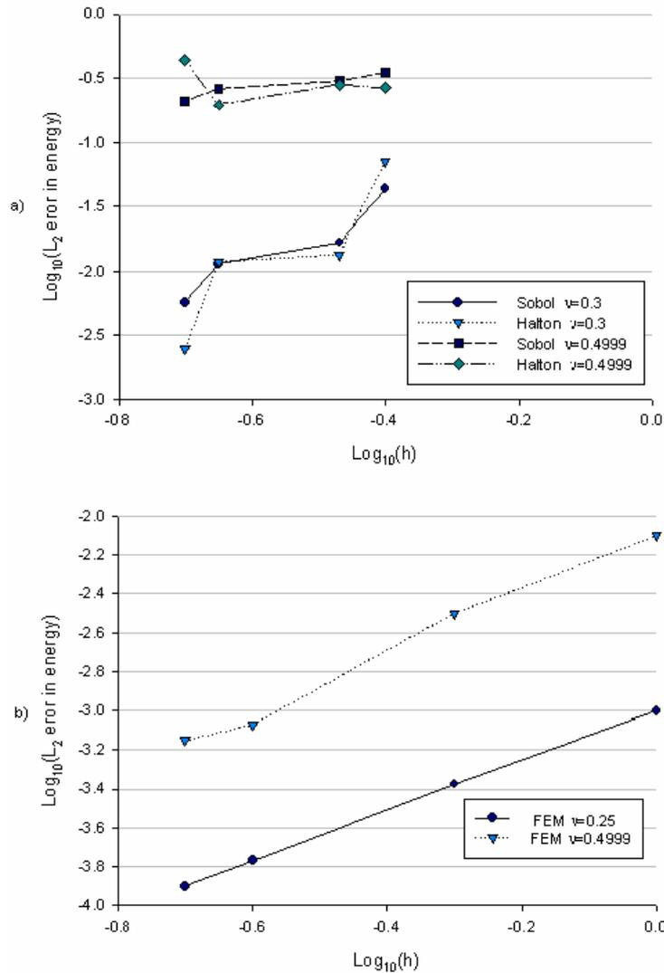
Figure 3: Convergence in strain energy obtained using Sobol and Halton quasi-random integration sequences. a) EFG method and b) Finite element method (using 9-noded displacement based finite element)
