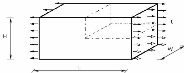
Figure 1: Uniform axial traction element: geometry and load
