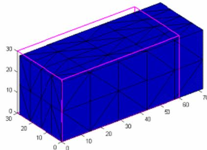
Figure 2: Deformed element subject to uniform axial loading
