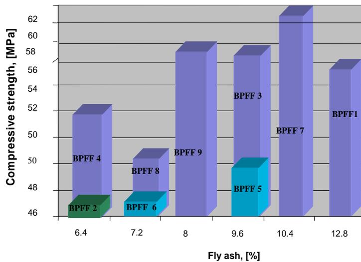
**Fig. 3.** – Variation of compressive strength for polymer concrete with fiber.
