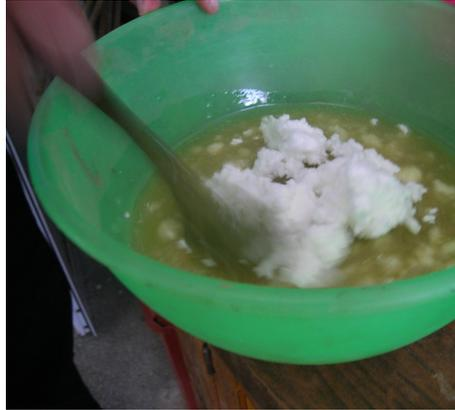
**Fig. 1.** – Cellulose fiber mixing with resin.
