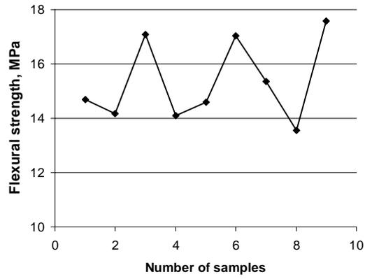
Fig. 6. – Variation of flexural strength for polymer concrete with fiber.
