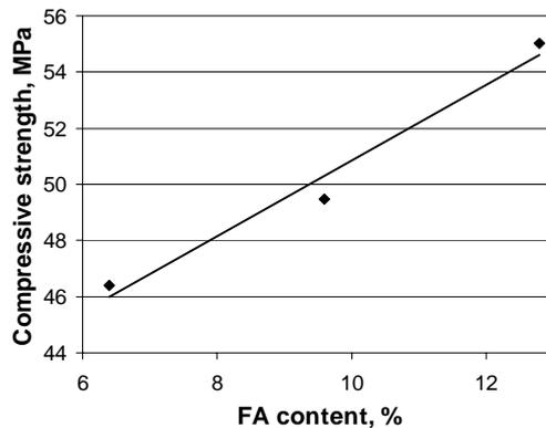
**Fig. 5.** – Variation of compressive strength for polymer concrete with fiber vs. the FA content, for 12.4% resin.
