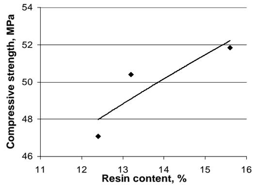
**Fig. 4.** – Variation of compressive strength for polymer concrete with fiber vs. the resin content, for 6.4% FA.
