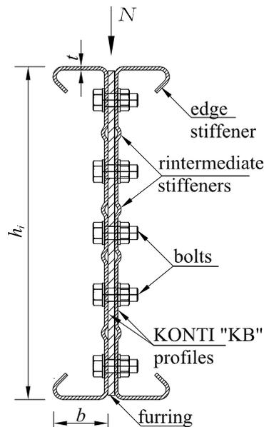
**Fig. 1.** – Cross section of the thin-walled type KB profiles.
