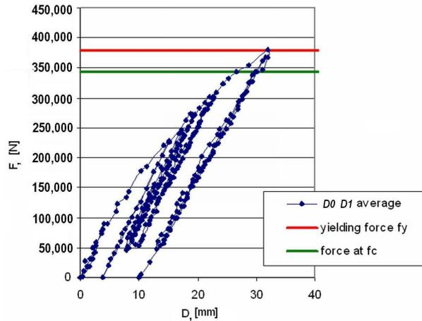
**Fig. 10.** – The force–deflection relationship at the midspan of the *N*-KB 600-5.0.
