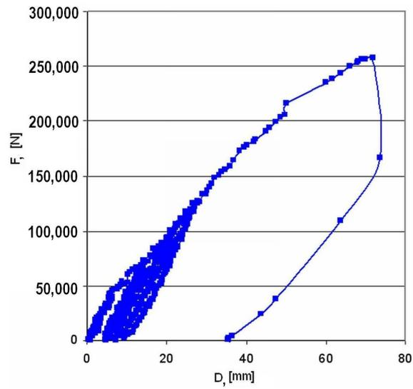
**Fig. 15.** – The force–deflection relationship (*D0-D1* average) for the *R*-KB 450-3.5 beam.
