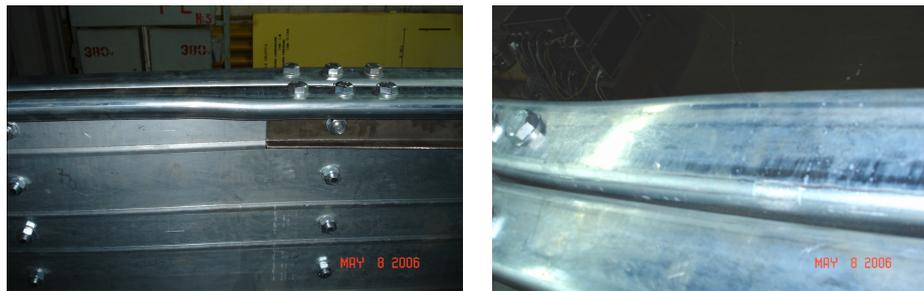
Fig. 12. – The local buckling of the KB element of the R-KB 600-5 beam.
