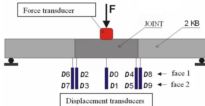
**Fig. 7.** – The transducer positions on the two sides of beams.
