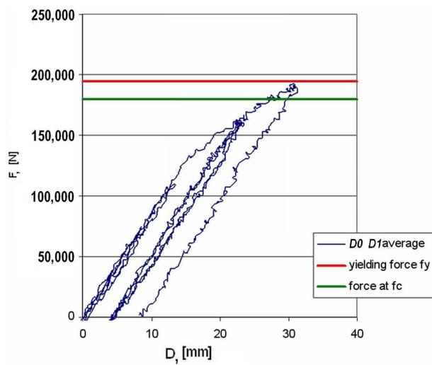
Fig. 13. – The force–deflection relationship at the midspan of the N-KB 450-3.5 beam.
