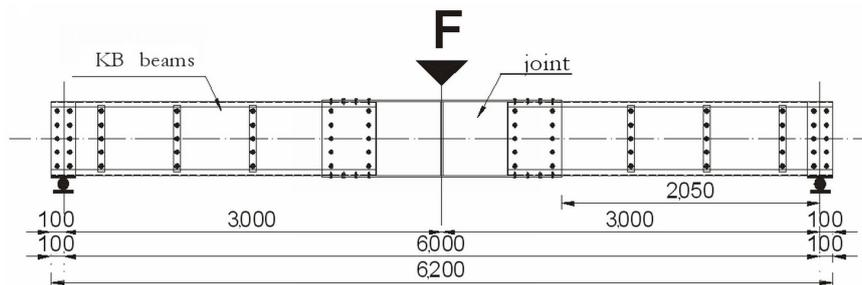
**Fig. 3.** – The dimensions of the proposed specimens.
