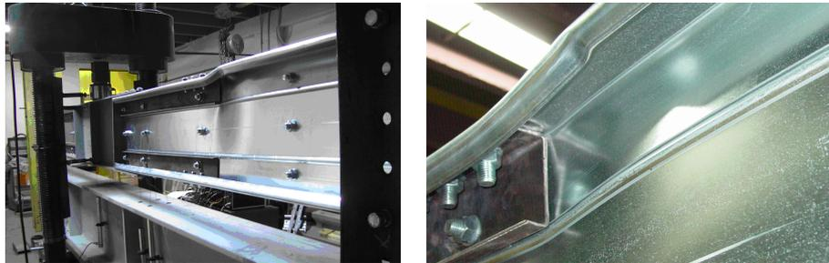
**Fig. 16.** – The local buckling of the KB element of the R-KB 600-5 beam.
