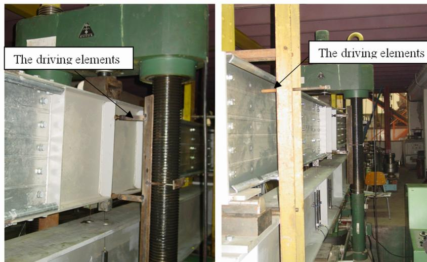
**Fig. 8.** – The driving elements mounted to prevent the lateral buckling.
