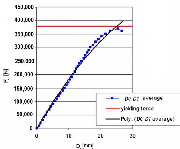
**Fig. 9.** – The force–deflection relationship at the midspan of the KB 600-5.0 beam.
