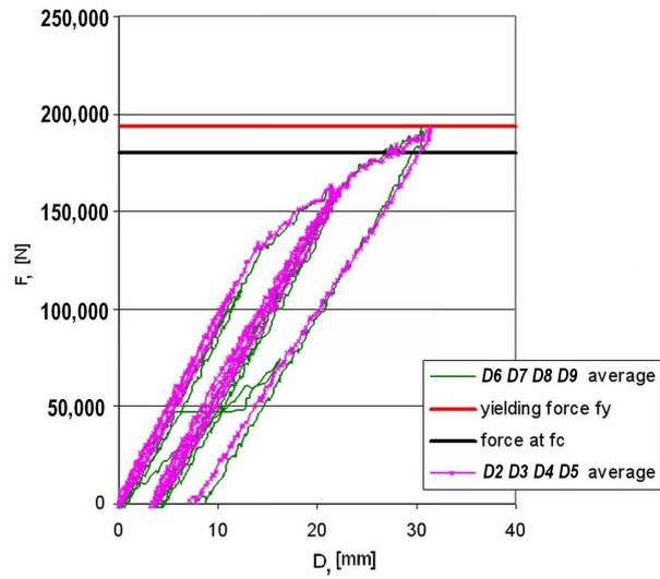
**Fig. 14.** – The force–deflection relationship at the joint ends for the *N*-KB 450-3.5 beam.
