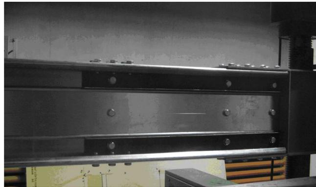
**Fig. 6.** – The positions of the strengthening elements R-KB 450-3.5.
