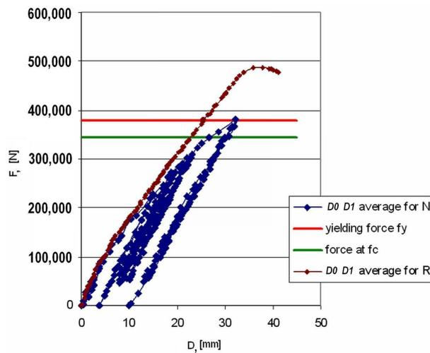
**Fig. 11.** – The force–deflection relationship for the *N*-KB 600-5.0 and *R*-KB 600-5.0 beams.
