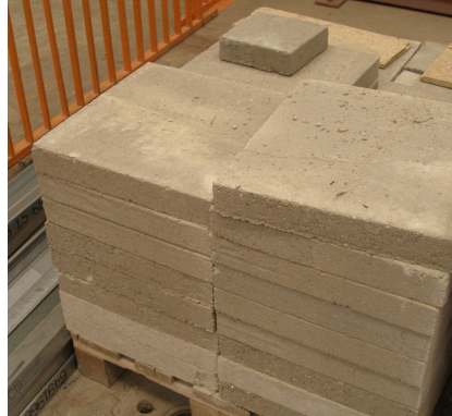
Fig. 4. – Additional weights for loading the structure.
