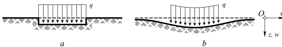
Fig. 1 – Deflections of elastic foundations under uniform pressure: a – Winkler foundation; b – practical soil foundations.
