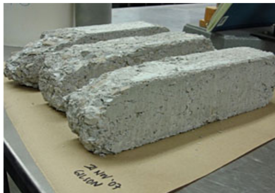
Fig. 5 – Exposing of aggregates.
