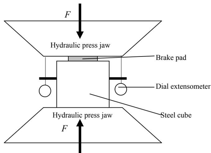
Fig. 3 – Device inserted between the press jaws.
