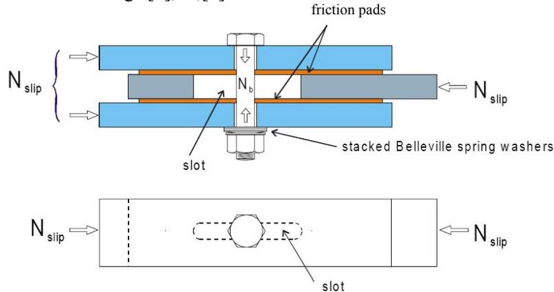
Fig. 1 – Basic slotted friction damper.
