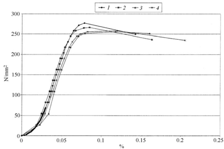
Fig. 6 – Behaviour curves for the friction material of the brake pads.
