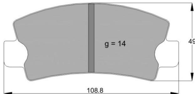
Fig. 2 – Tested brake pad layout.
