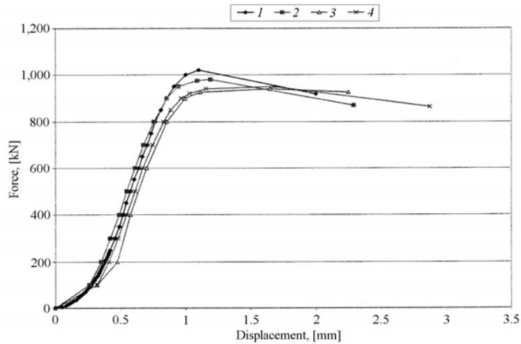
Fig. 5 – Compression behaviour for the friction material of the brake pads.
