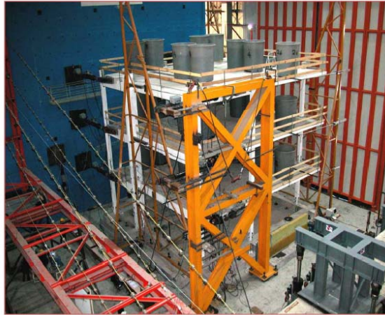
Fig. 2. – Pseudo-Dynamic testing facility at Joint Research Center (Photo courtesy of Francisco J. Molina, Ph.D. [16]).
