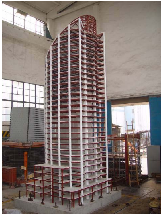
Fig. 3. – Scale model of the LG Beijing tower, shaking table test facility at Tongji University, China (Photo courtesy of Wensheng Lu, Ph.D. [17]).
