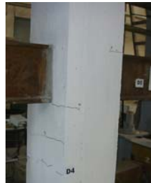
Fig. 13 – Failure mechanism of the steel concrete composite joint asymmetrical load: a – distribution of cracks at the composite steel concrete joint asymmetrical load test; b – distribution of first cracks in joint and column; c – cracks distribution at failure.
