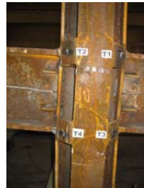
Fig. 12 – Failure mechanism of the steel joint asymmetrical load: a – general view of steel joint – asymmetrical load; b – tearing of vertical stiffener; c – general view of joint at failure.
