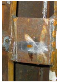
Fig. 12 – Failure mechanism of the steel joint asymmetrical load: a – general view of steel joint – asymmetrical load; b – tearing of vertical stiffener; c – general view of joint at failure.
