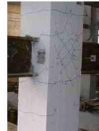
Fig. 13 – Failure mechanism of the steel concrete composite joint asymmetrical load: a – distribution of cracks at the composite steel concrete joint asymmetrical load test; b – distribution of first cracks in joint and column; c – cracks distribution at failure.
