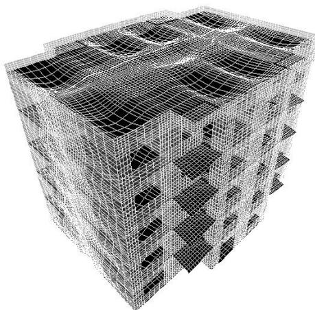
Fig. 5 – The deformed shape of the structure due to the 861IAS2 seismic action.
