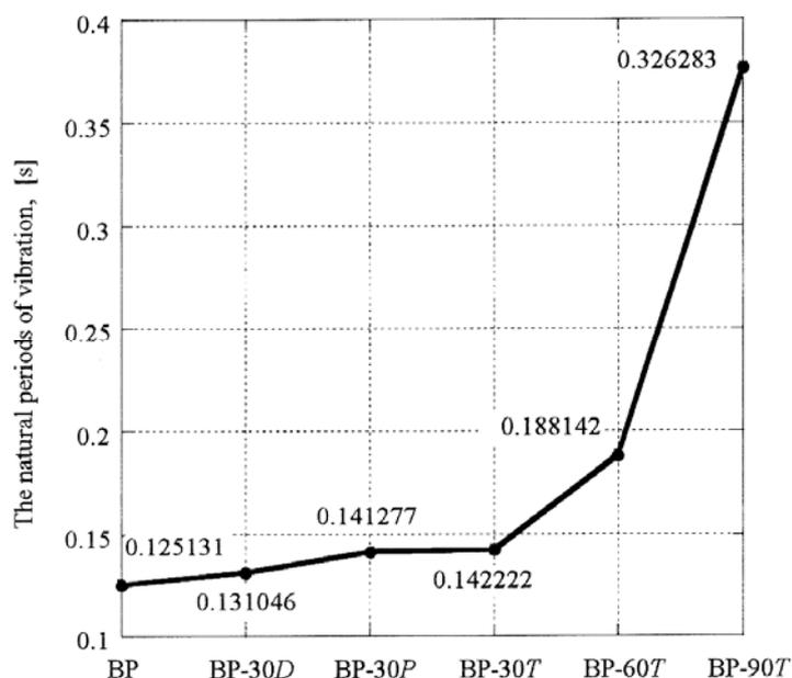
Fig. 6 – The variation of the first natural period of vibration due to the position and the degradation percentage of the affected elements of the building.
