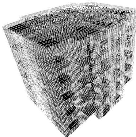
Fig. 4 – The deformed shape of the structure corresponding to the first mode of vibration with  $T = 0.125131$  s.
