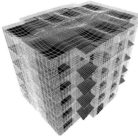
Fig. 3 – The deformed shape of the structure due to the self weight.
