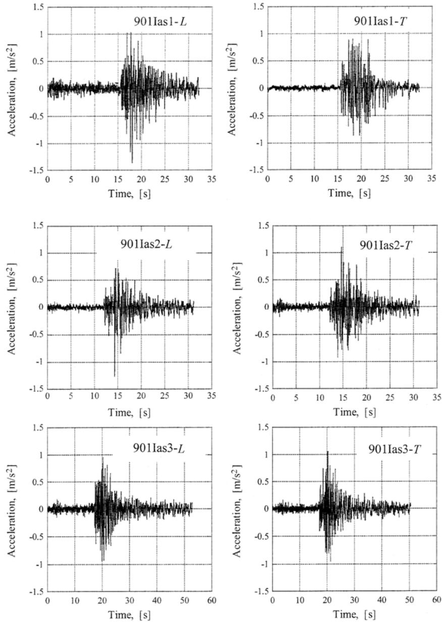
Fig. 2 – The Acceleration diagrams for 1990 Vrancea Earthquake recorded at the stations IAS1, IAS2 and IAS3 (the longitudinal component,  $L$ ; the transversal component,  $T$ ).
