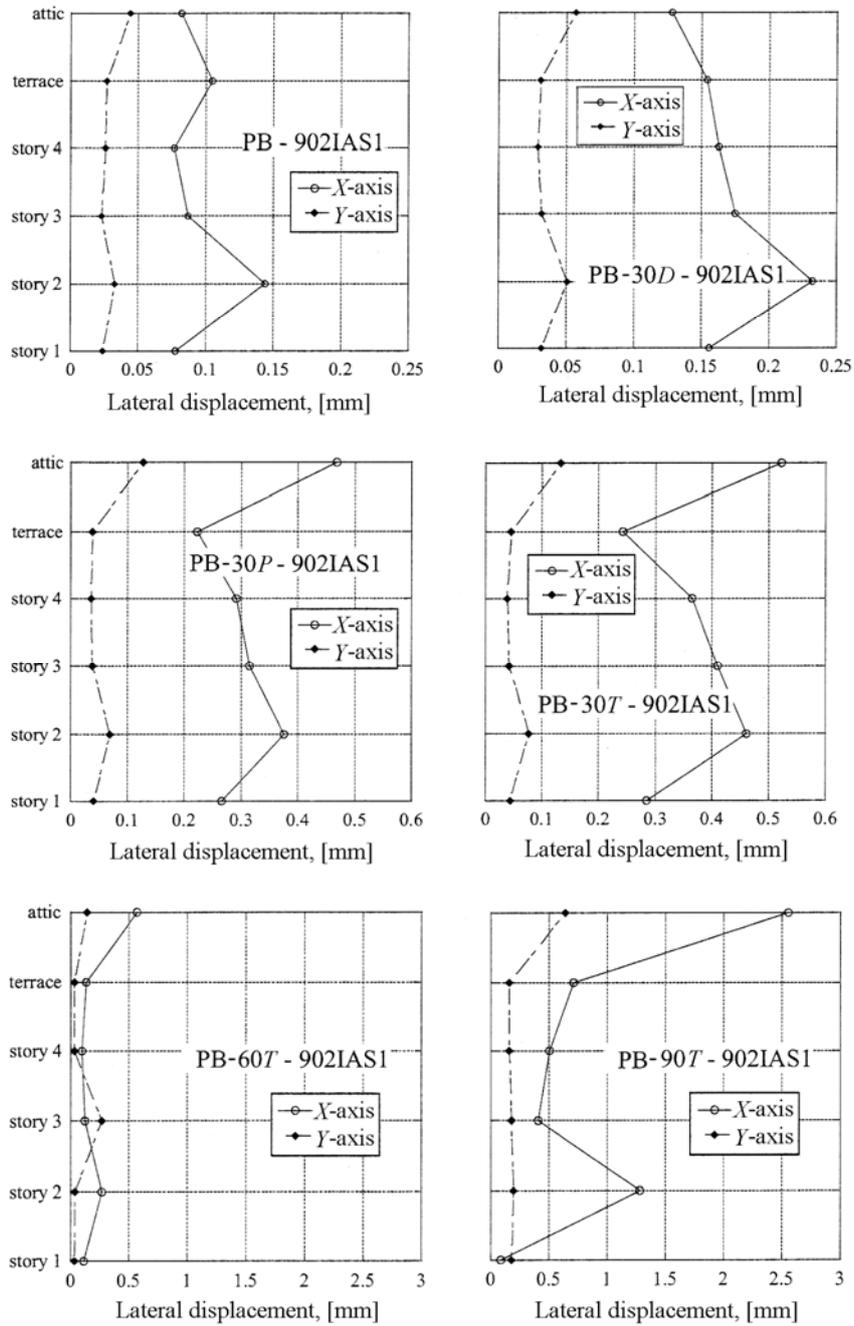
Fig. 8 – The lateral displacements of the structure due to the 902IAS1 seismic action.
