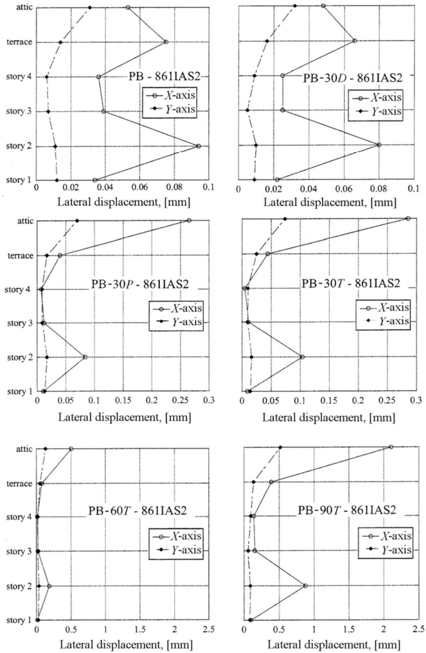
Fig 7 – The lateral displacements of the structure due to the 861IAS2 seismic action.
