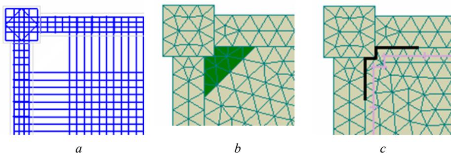
Fig. 6 – Studied cases: *a* – reduced reinforcement; *b* – material replacement in the corners; *c* – 5 mm joint in the corners.
