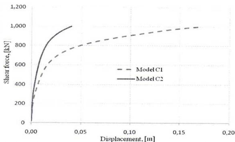
Fig. 9 – Capacity curves for frame without slab and frame with slab.
