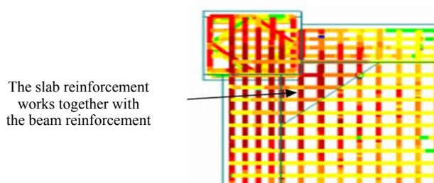
Fig. 5 – Slab influence on potential plastic areas from the beams.
