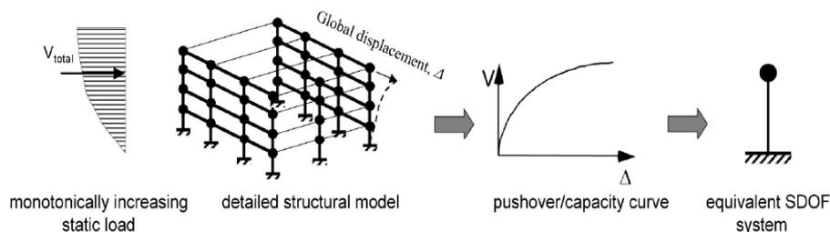
Fig.1 – Schematics depicting the development of an equivalent SDOF system for a pushover curve (FEMA 440, 2005).
