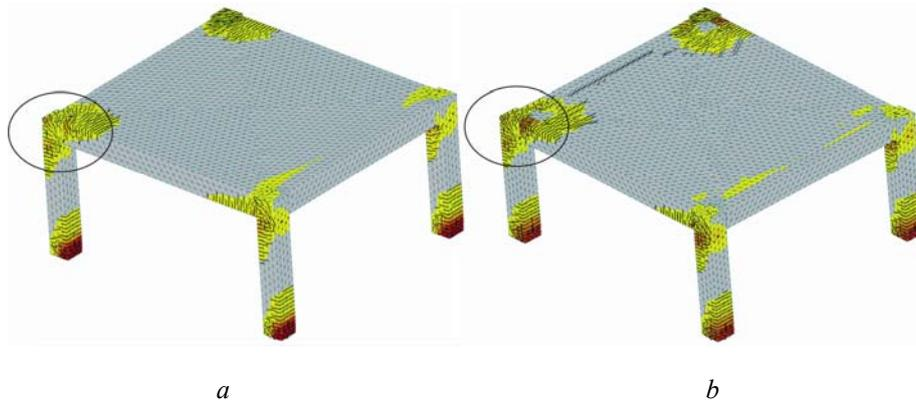
Fig. 7 – Plastic hinge development: *a* – model C2; *b* – model C6.
