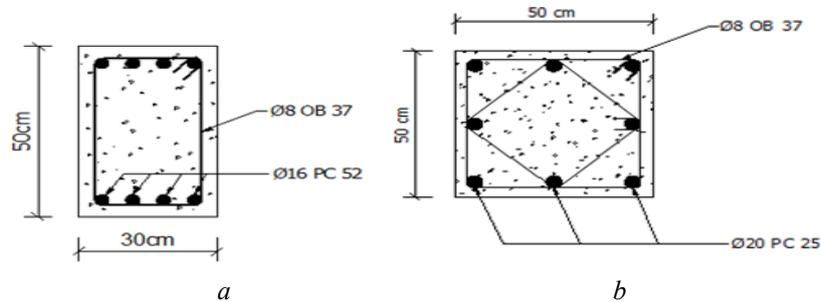
Fig. 4 – Considered cross-sections: *a* – beams; *b* – columns.
