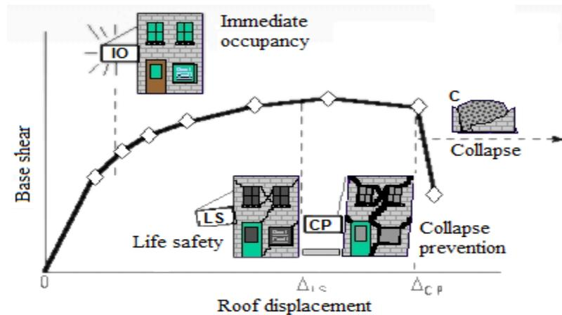
Fig. 2 – Pushover curve and structural performance stages.
