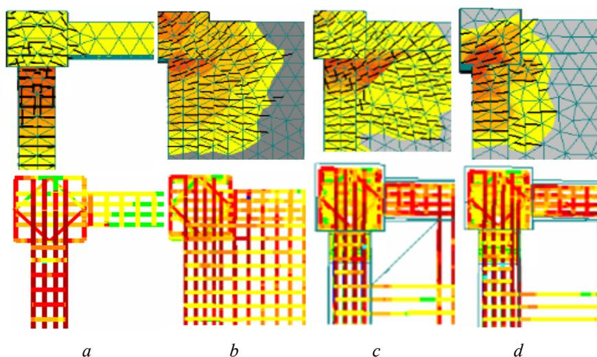
Fig. 8 Cracks and stress development for : *a* – model *C1*;
