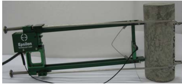
Fig. 6 – Positioning of the longitudinal extensometer.
