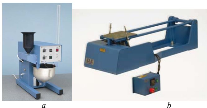
Fig. 1 – The automatic mixer (a) and the shock machine (b) utilized to manufacture test samples.
