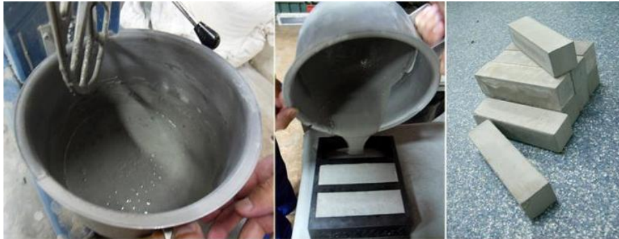
Fig. 2 – Preparing the samples for tensile and compressive testing.
