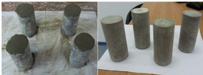
Fig. 3 – Preparing the samples to determine Young's modulus and Poisson's ratio.
