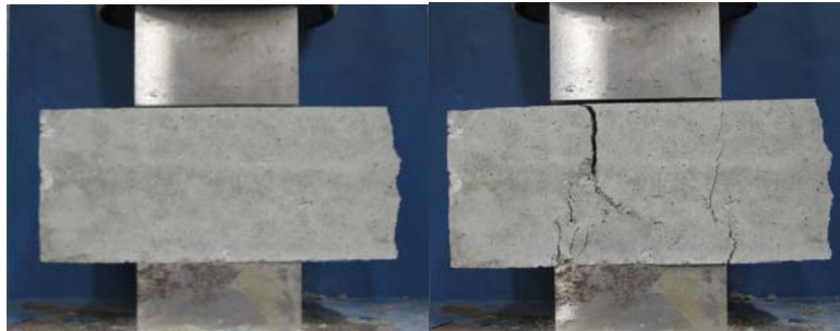
Fig. 5 – Compressive testing of prismatic sample.
