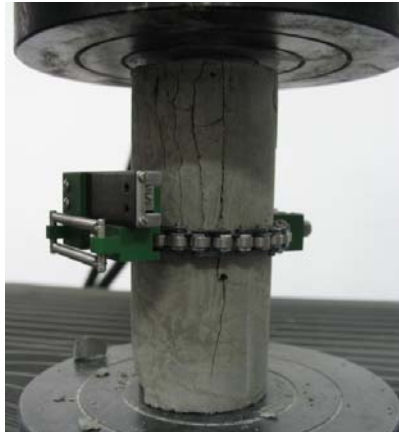
Fig. 7 – Tested cylinder with circumferential extensometer.
