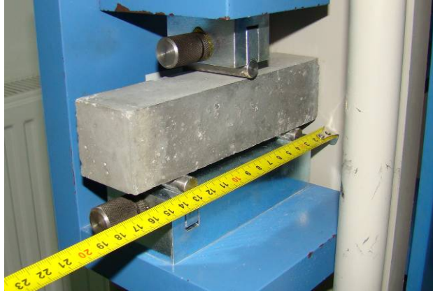
Fig. 9 – 160 × 40 × 40 mm prism tested in bending.
