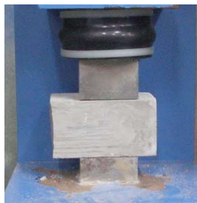
Fig. 2 – Uniaxial compression test on a half prism.
