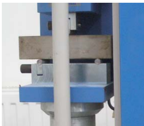
Fig. 1 – Three-point bending test of mortar prism.
