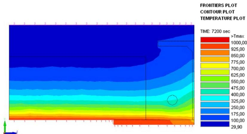
Fig. 3 – Temperature distribution on the cross-section after two hours of ISO fire.
