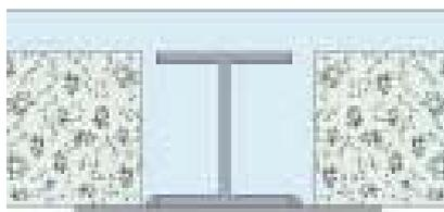
Fig. 1 – Slim Floor system – steel beam supporting prefabricated elements.
