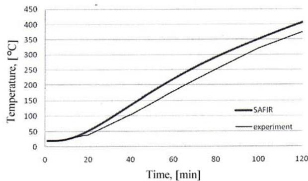
Fig. 5 – Temperature in rebars.
