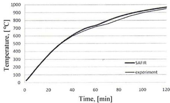
Fig. 4 – Temperature evolution in the bottom flange.
