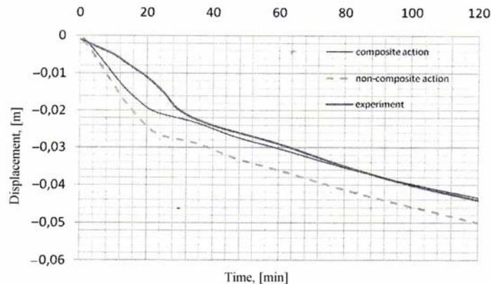
Fig. 6 – Displacement evolution at mid-span of the floor.
