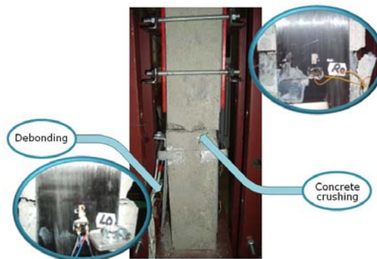
Fig. 7 – Typical failure mode.
