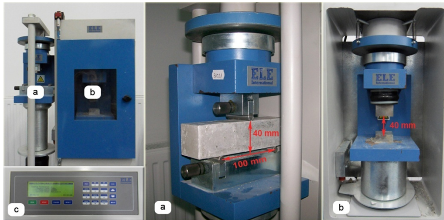
Fig. 4 – Compression and bending test equipment: a – bending; b – compression; c – testing equipment computer.
