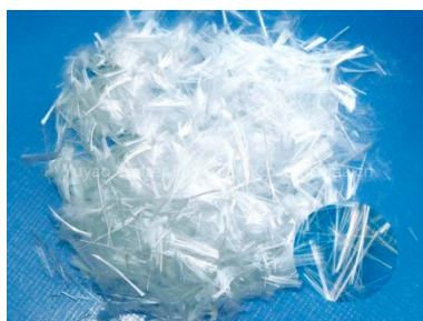
Fig. 3 – Short polypropylene fibers used for mineral matrix reinforcement.
