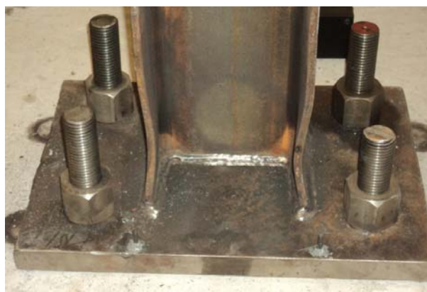
Fig. 10 –Plastic hinge formation in the column.
