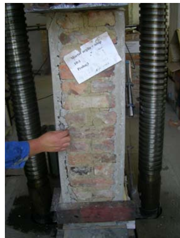
Fig. 13 – Fracture in polymer grid reinforced coating.
