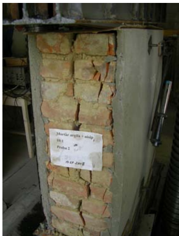
Fig. 12 – Fracture in steel grid reinforced coating.
