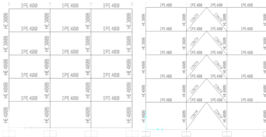
Fig. 2 – Unbraced and braced steel frame.
