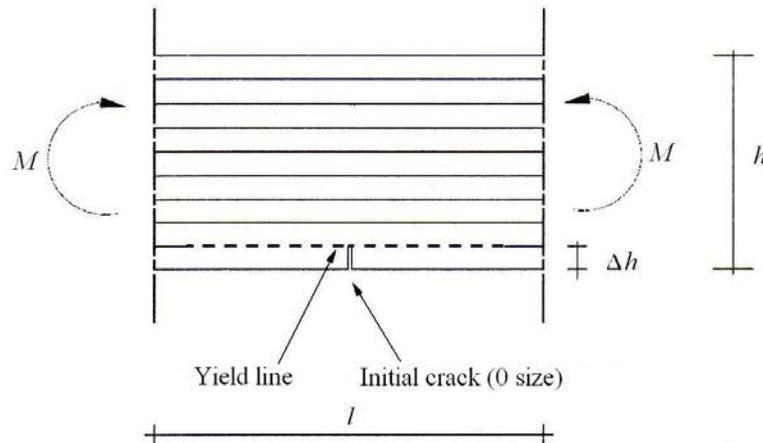
Fig. 1 – The laminated beam, having an initial crack with a length equal to the laminating line thickness; the dotted line represents the crack propagation direction.
