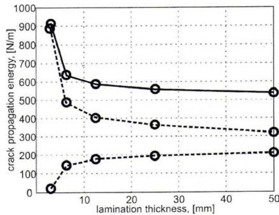
Fig. 7 – Energy consumption for the propagation of a fully developed (solid line) fracture area with various laminated thicknesses; the discontinuous line shows the contribution of mode I and the dotted line the contribution of mode II.
