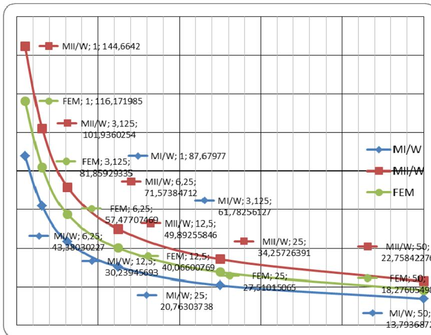
Fig. 3 – Bending resistance ( $M/W$ ), compared to laminated thickness for a beam having 450 mm height; the circles are results of FEM simulations. The lines with squares and diamonds are determined based on eq. (1) for  $G_c = G_{Ic}$  (diamonds) and  $G_c = G_{IIc}$  (squares).
