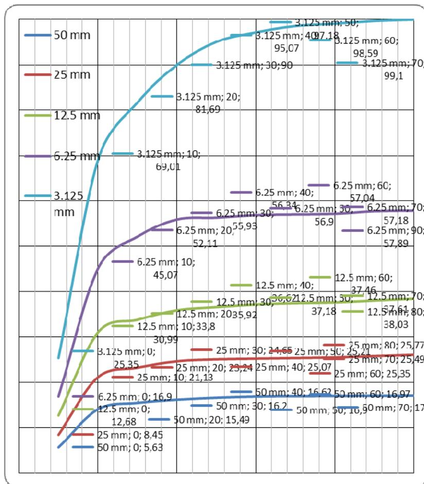
Fig. 4 – Unitary bending stresses ( $MW$ ), vs. tip crack position for different laminate thicknesses.
