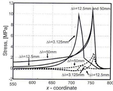
Fig. 5 – Stress distribution along the fixture line of ultra-peripheral laminates having top load; continuous lines show shearing stress and the discontinuous line shows normal stress.
