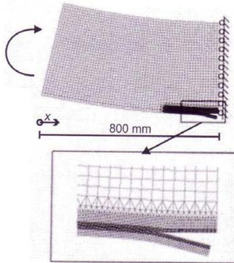
Fig. 2 – The deformed beam at maximum load; the crack has expanded by 50...60 mm.
