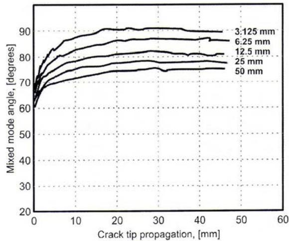
Fig. 6 –  $\phi$  angle for mixed yielding modes, as defined in eq. (2), vs. the crack tip position for laminates having different thicknesses.
