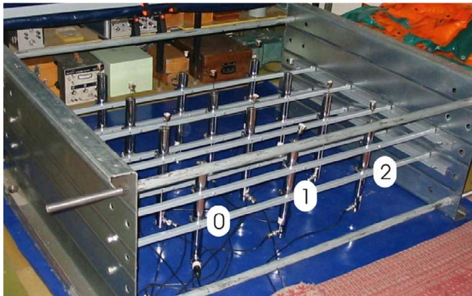
Fig. 2 – The testing stand with the inductive transducers.
