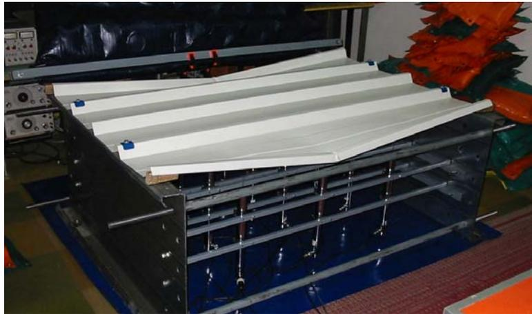
Fig. 4 – The collapse of the E3-050 specimen (buckling).
