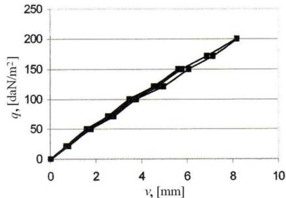
Fig. 3 – The measured displacement at the midspan of the E2-05 specimen.
