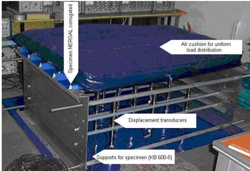
Fig. 1 – View of the testing stand.
