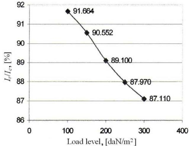
Fig. 6 – The dependence of stiffness characteristic vs. load level (0.75 mm steel sheet).
