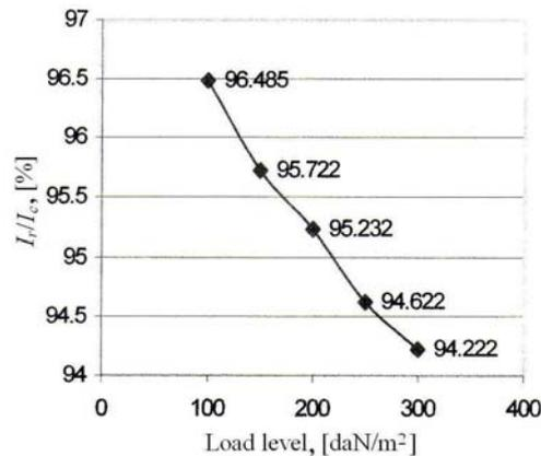
Fig. 8 – The stiffness characteristic vs. load level dependence (1 mm thickness sheet).
