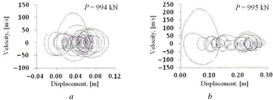
Fig. 13 – Phase-plane: *a* – stable motion; *b* – unstable motion.
