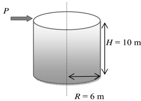
Fig. 11 – Example of the cylindrical tank under a concentrated load at the top.
