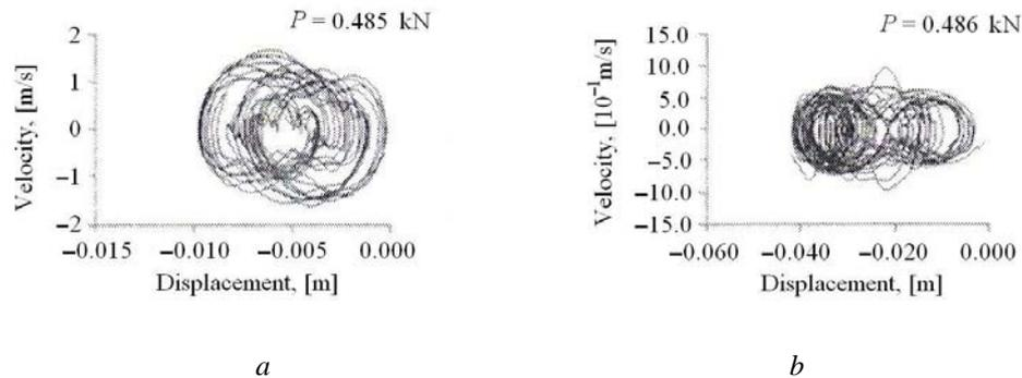
Fig. 10 – Phase-plane: *a* – stable pre-buckling motion; *b* – stable post-buckling motion.
