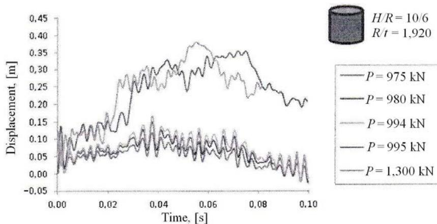
Fig. 12 – Dynamic response of the radial displacement at the top of tank.
