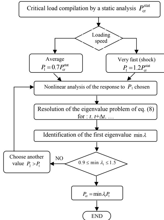
Fig. 7 – Schematic application of the pseudo-dynamic method.
