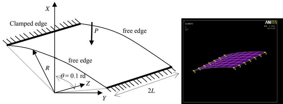
Fig. 8 – Example of a cylindrical roof under concentrated load.
