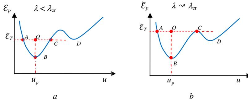
Fig. 2 – Variation of potential energy as a function of some displacement variable:
