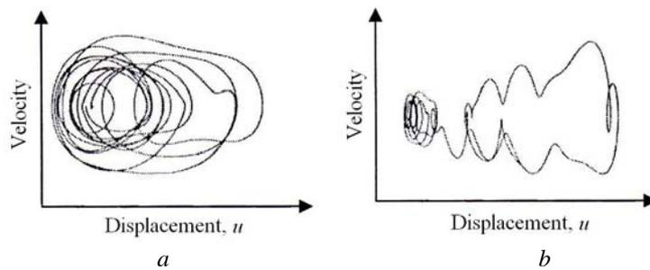
Fig. 1 – Phase plane: a – stable motion; b – unstable motion.
