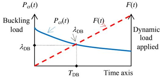
Fig. 6 – Critical load determined by the geometric process.
