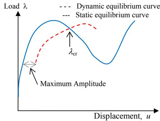
Fig. 3 – Critical load factor at the intersection of the two curves of static and dynamic equilibrium.
