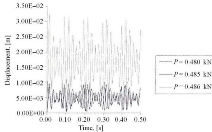
Fig. 9 – Dynamic response of the center of the cylindrical roof.
