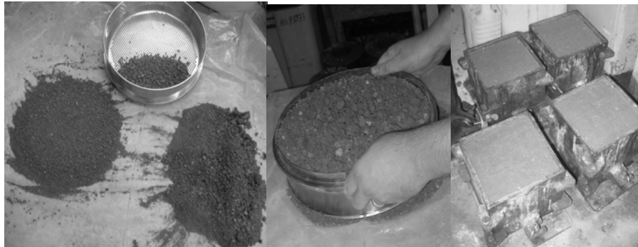
Fig. 1 – The earth is sifted and rammed into metal moulds.
