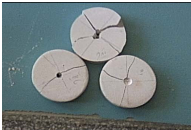
Fig. 3 – Fracture of plaster disks.
