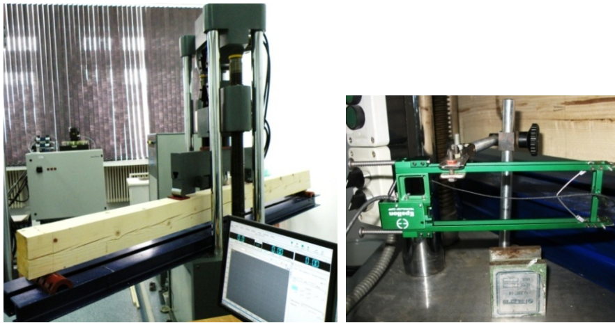
Fig. 4 – Test equipment and arrangements for the four-point bending test.
