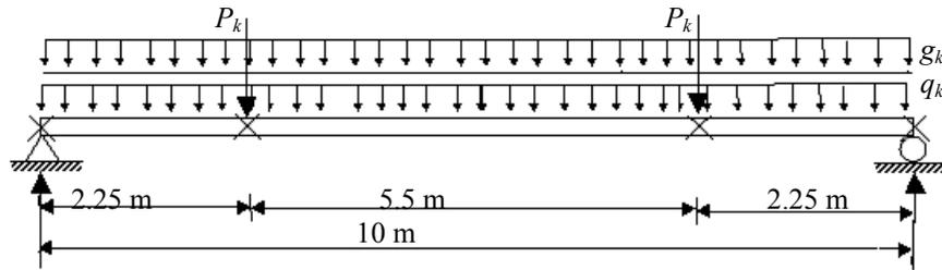
Fig. 4 – Variable imposed load and the span of the composite I beam floor system.
