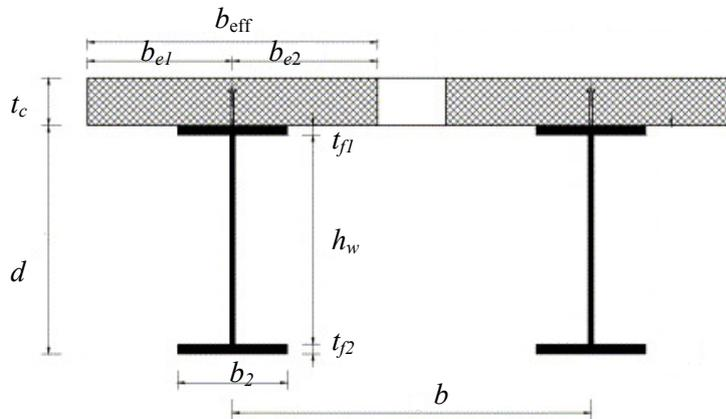
Fig. 1 – Notations for composite I welded beam.
