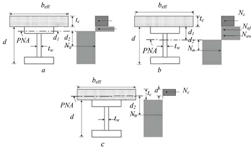
Fig. 2 – Plastic design of composite beam: a – when *PNA* lies in steel flange;
