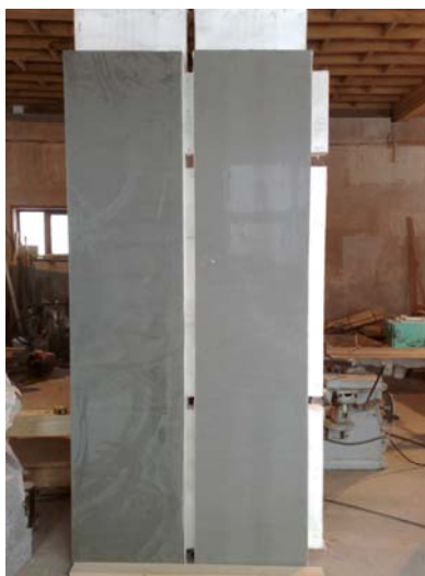
Fig. 2 – Prototype of the wall panels made of GFR mineral matrix.
