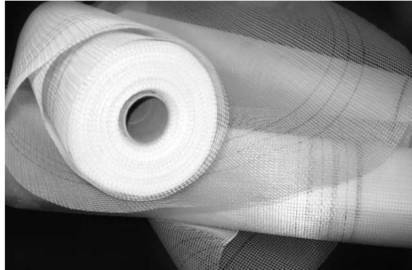
Fig. 3 – Glass fiber fabric used in matrix reinforcement.
