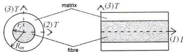
Fig. 6 – Self-consistent model.
