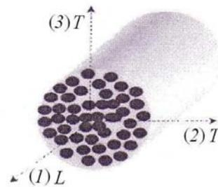
Fig. 2 – A unidirectional fibre reinforced round bar and its principal axes.
