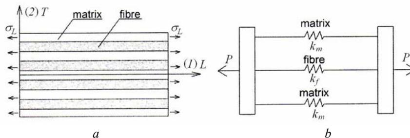
Fig. 3 – Model for FRP composite for predicting composite behaviour: *a* – composite lamina constituents; *b* – parallel model.
