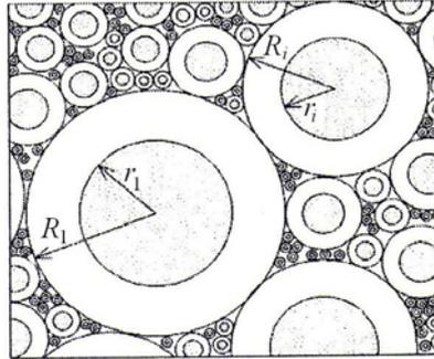
Fig. 5 – Composite cylinder assemblage (CCA).
