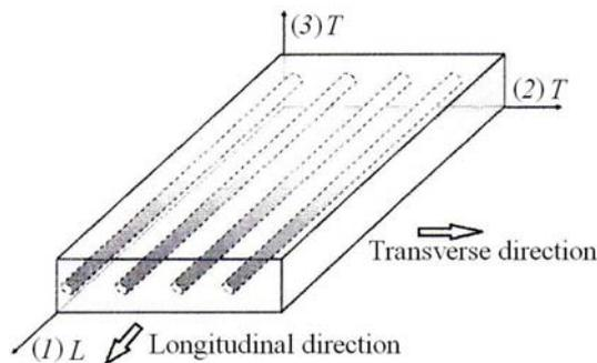
Fig. 1 – A unidirectional fibre reinforced lamina and principal material axes.
