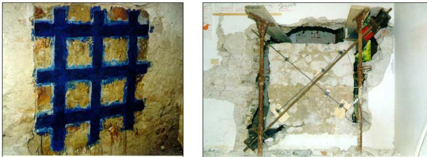
Fig. 3 – Reinforcing masonry with unidirectional carbon/glass fibers sheets and layout of diagonal compression tests (Borri *et al.*, 2003).
