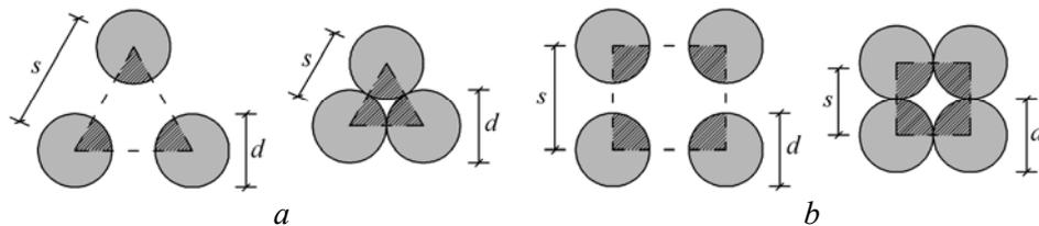
Fig. 3 – Representative area elements for idealized fibre- packing geometries
