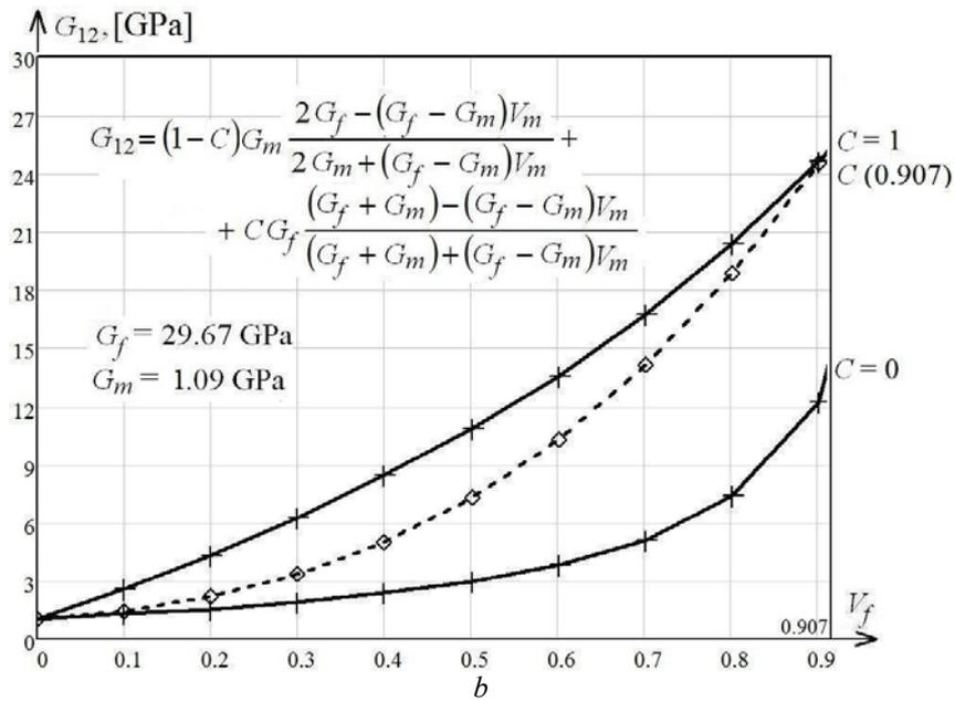
Fig. 7 – Variation of shear modulus including the influence of fibres contiguity:  $a$  – averaging factor  $C_{0.785}$ ;  $b$  – averaging factor  $C_{0.907}$
