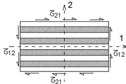
Fig. 5 – The model used for the shear elastic modulus analytical evaluation.
