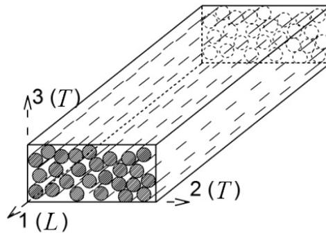
Fig. 1 – A unidirectional fibre reinforced lamina with its principal material axes.
