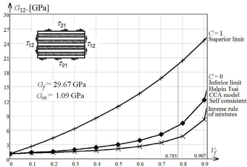
Fig. 12 – Synthesis of all results for the transverse modulus.
