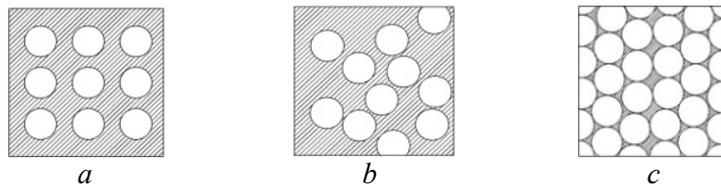
Fig. 4 – Various schemes of fibre contiguity: *a* – isolated fibres ( $C = 0$ ); *b* – actual random fibre ( $0 < C < 1$ ); *c* – isolated matrix ( $C = 1$ ).
