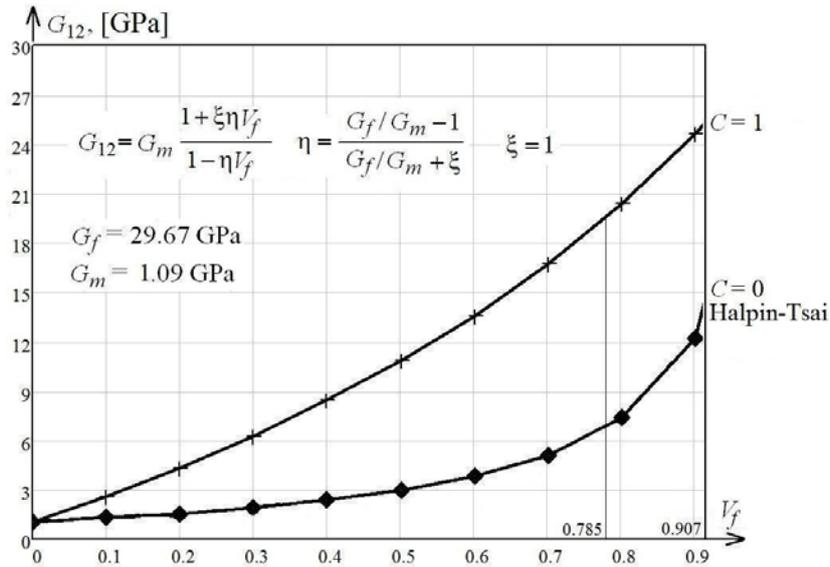
Fig. 9 – Shear modulus predicted through Halpin-Tsai equations *versus* influence of contiguity factor.
