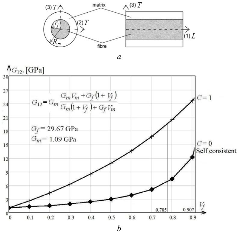
Fig. 11 – Self-consistent model: *a* – the constituents assemblage; *b* – variation of shear modulus with fibre content.
