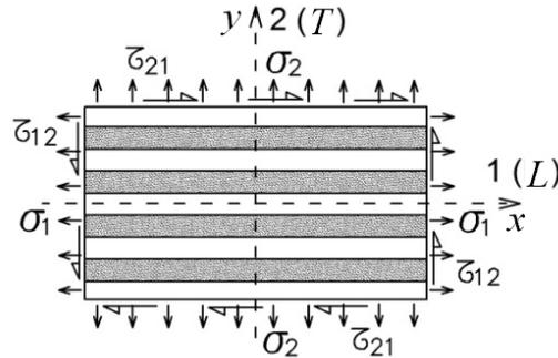
Fig. 2 – Specially orthotropic lamina under plane state of stress.
