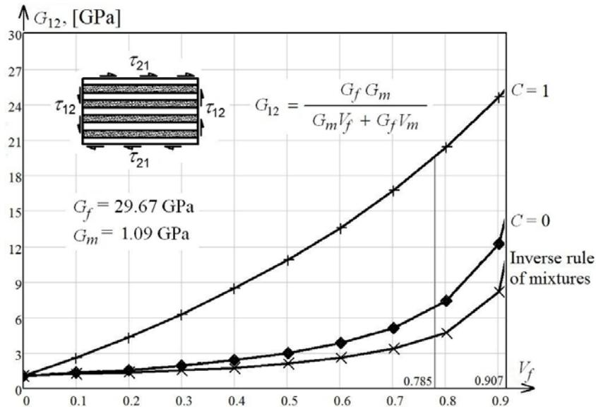
Fig. 6 – Variation of  $G_{12}$  by inverse rule of mixtures compared to extreme contiguity.
