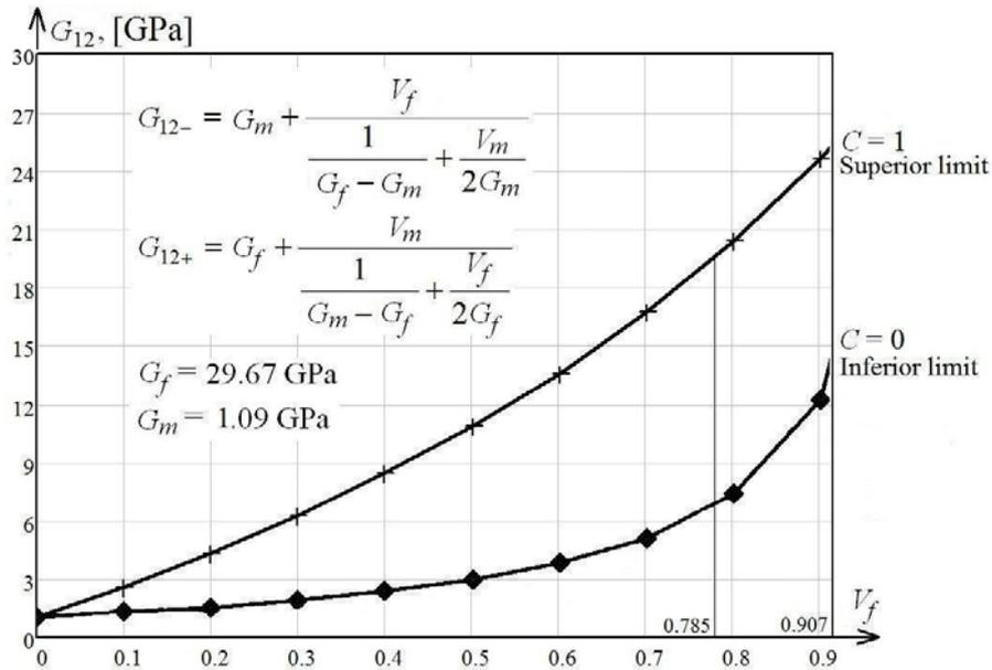
Fig. 8 – Superior and inferior limits for shear modulus.
