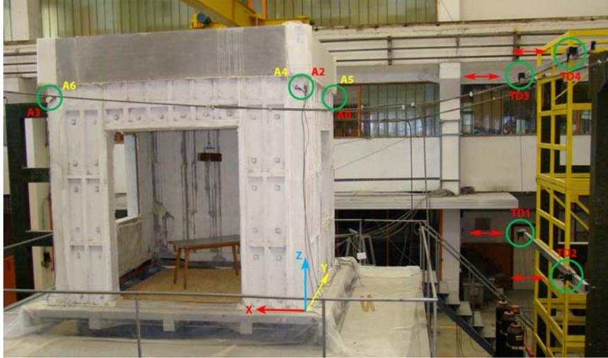
Fig. 7 – Placement of the transducers on the experimental model: A0, A1, A2, A3 – accelerometers on X-direction; A4, A5, A6, A7 – accelerometers on Y-direction; TD1, TD2, TD3, TD4 – displacement transducers.
