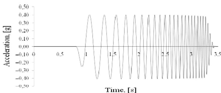
Fig. 10 – Gliding sinus type accelerogram.
