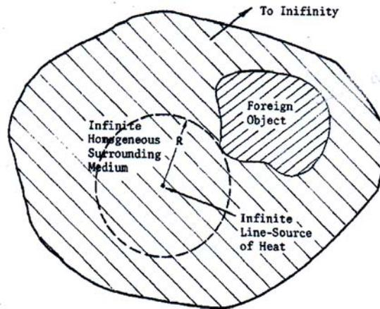
Fig. 2 – Probe non-uniformity interaction pattern.
