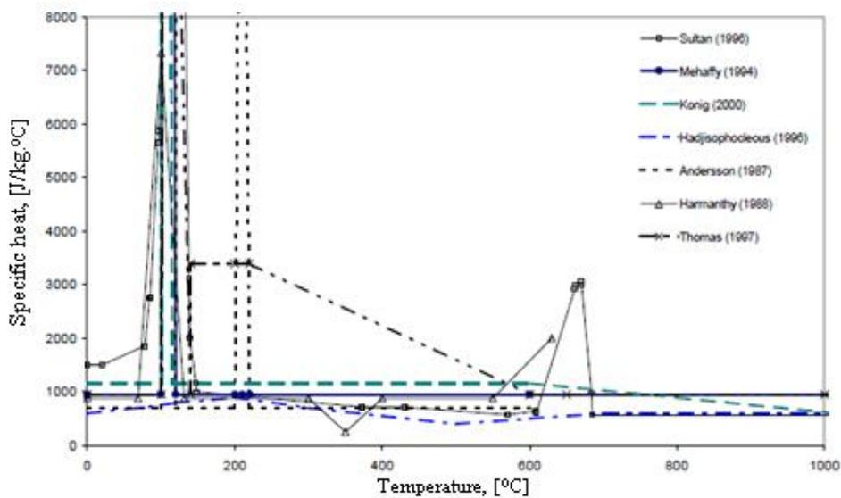
Fig. 5 – Specific heat of gypsum boards according to various researchers.
