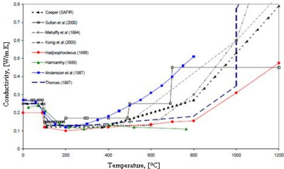
Fig. 7 – Thermal conductivity of gypsum *versus* temperature.
