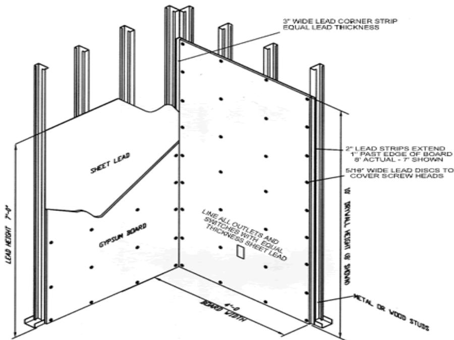
Fig. 1 – A typical gypsum board wall assembly.
