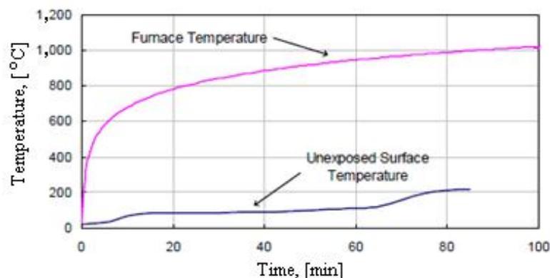
Fig. 2 – Temperature development on the unexposed side of a gypsum board with 25 mm thickness subjected to a standard cellulosic fire.
