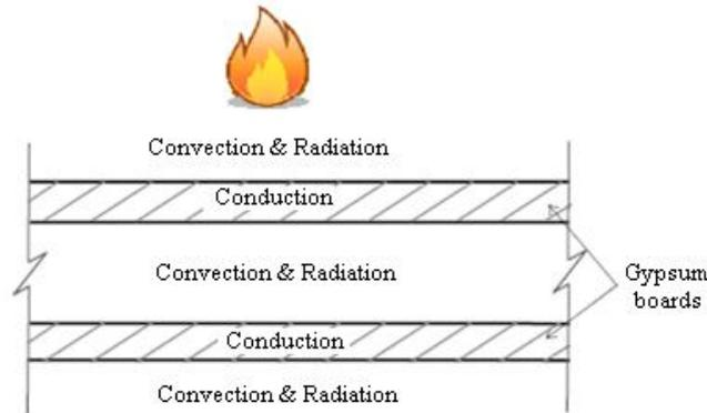
Fig. 4 – Heat transfer modes through gypsum board assemblies.
