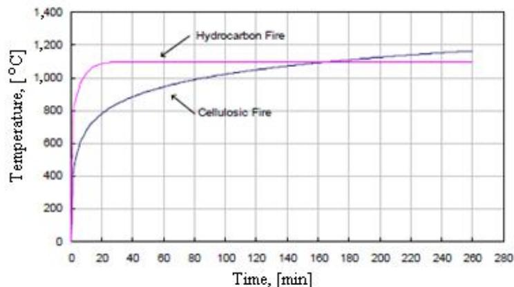
Fig. 3 – Time vs. temperature curves for standard fires according to BS476 (1987).
