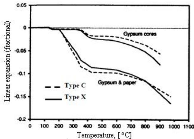
Fig. 9 – Contraction of gypsum as a function of temperature (Mehaffey *et al.*, 1994).
