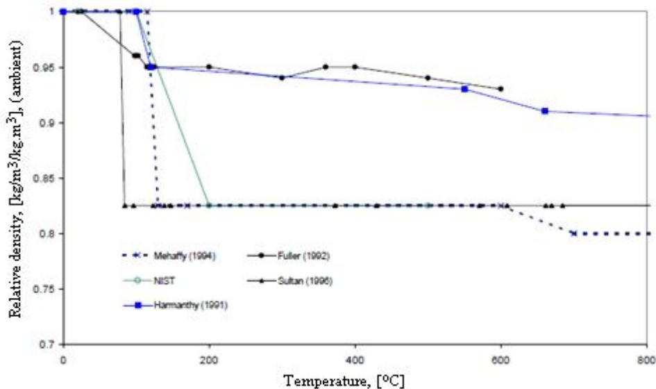
Fig. 6 – Density of gypsum board relative to ambient density, *versus* temperature.
