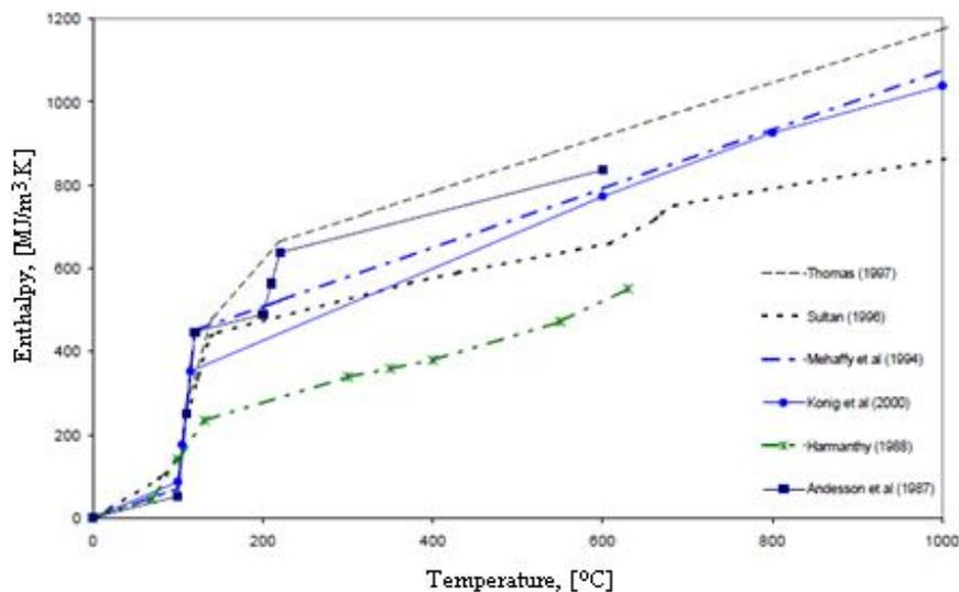
Fig. 8 – Comparative enthalpy of gypsum board from various sources.
