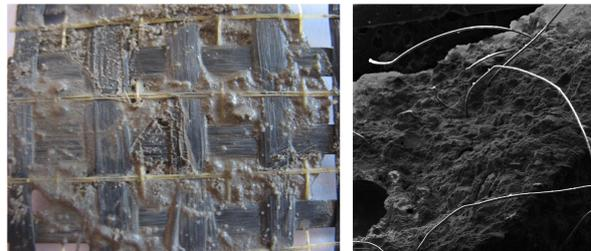
Fig. 2 – Optical and scanning electrons microscope images of double reinforced mineral matrix composites.
