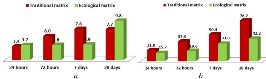
Fig. 11 – Experimental results of mechanical testing of traditional and ecological mineral matrix, [MPa]: *a* – tensile strength; *b* – compressive strength.
