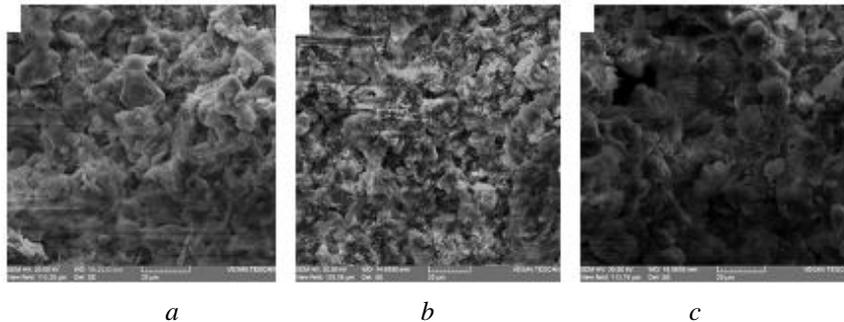
Fig. 8 – Microstructure of sample 2 at: *a* – 24 hours; *b* – 7 days; *c* – 28 days.
