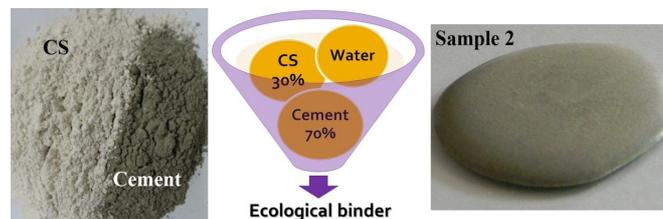
Fig. 5 *b* – Calcium sulphate and cement binder.
