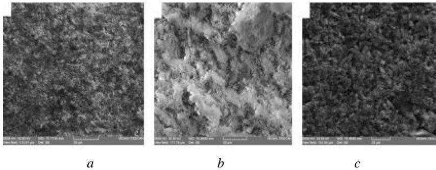
Fig. 7 – Microstructure of sample 1 at: *a* – 24 hours; *b* – 7 days; *c* – 28 days.
