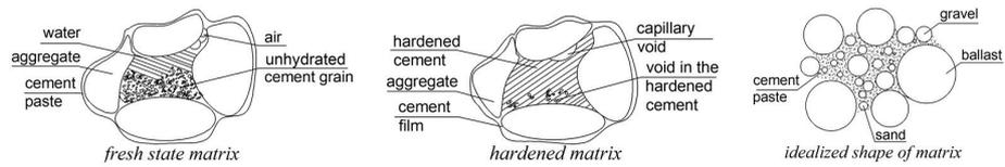
Fig. 1 – Simple reinforced composite with mineral matrix.
