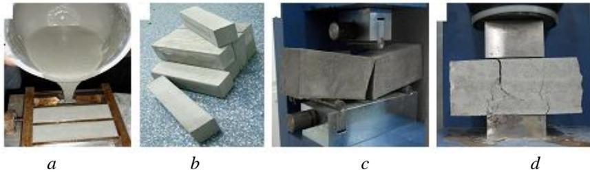
Fig. 10 – Preparation and testing of samples: *a* – samples casting; *b* – prismatic samples; *c* – bending test; *d* – compression test.
