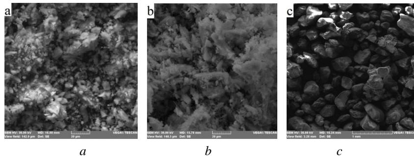
Fig. 6 – Microstructure of unhydrated elements: *a* – cement; *b* – CS; *c* – sand.
