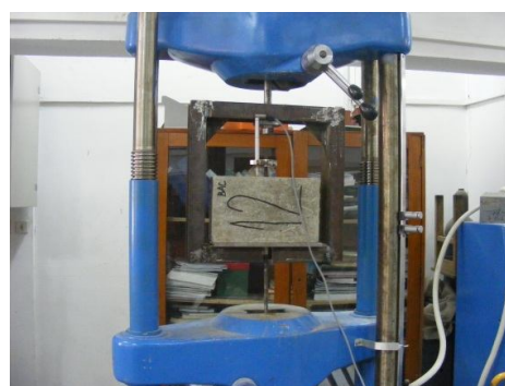
Fig. 4 – Test specimen prepared for pull-out test.
