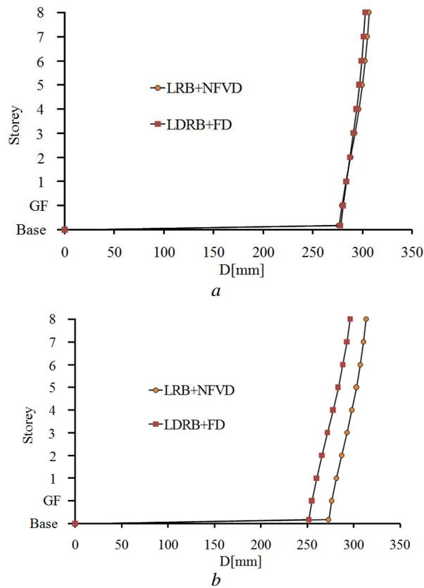
Fig. 2 – The mean relative displacements of the isolated structure, with LRB+NFVD and LDRB+FD system:  $a$  –  $x$ -direction;  $b$  –  $y$ -direction.
