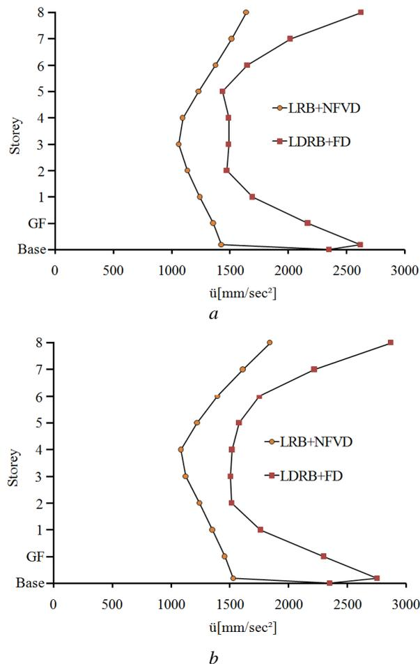
Fig. 3 – The mean absolute accelerations of the isolated structure, with LRB+NFVD and LDRB+FD system:  $a$  –  $x$ -direction;  $b$  –  $y$ -direction.
