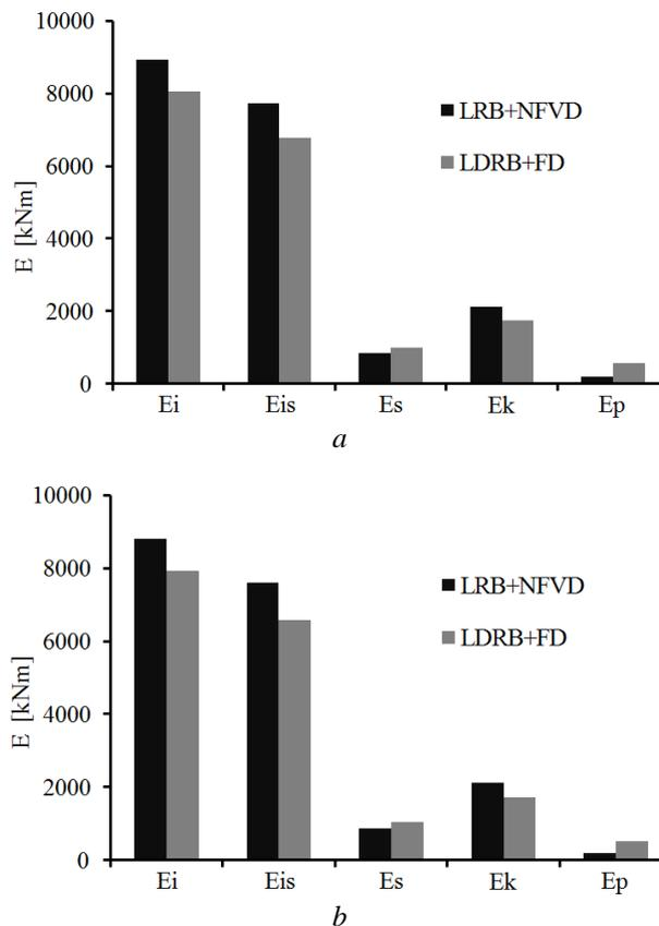
Fig. 4 – The mean energies of the two isolation system:
