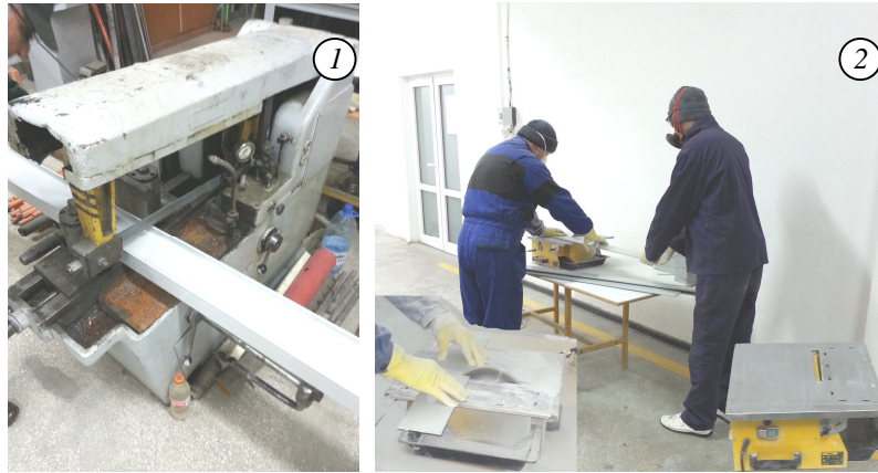
Fig. 6 – Specimens cutting: 1 – I-beams; 2 – plates.
