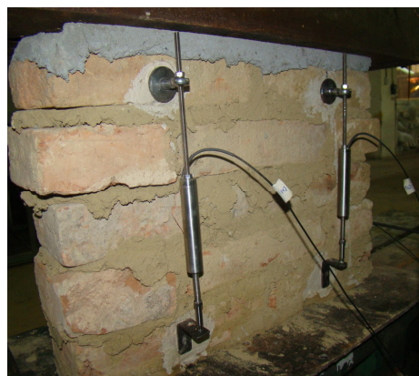
Fig. 9 – Control sample equipped with displacement traducers (on both sides).
