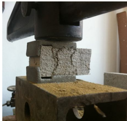
Fig. 7 – Determination of compressive strength of hardened mortar prisms.
