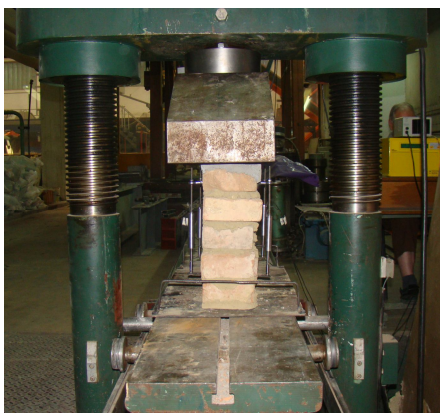
Fig. 8 – Handling of samples for testing at centric compression.
