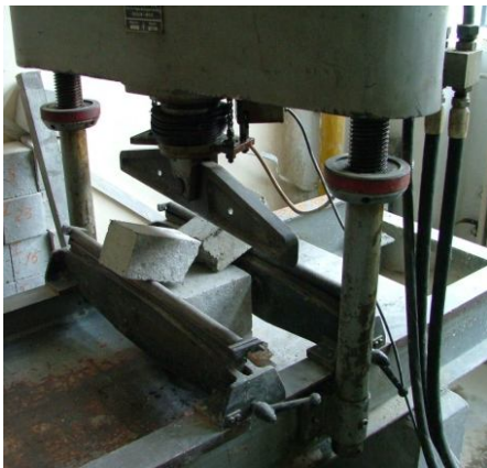
Fig. 6 – Reinforced mortar prism samples tested for tensile strength in bending.
