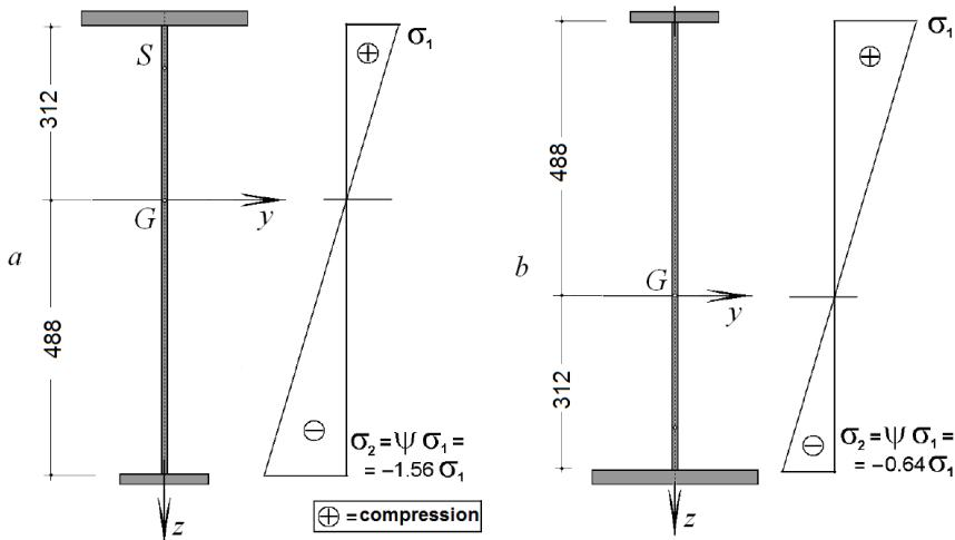
Fig. 2 – Evaluation of Cross – section class.
