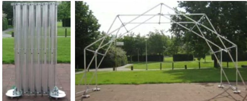
Fig. 4 – Kinetic arch before and after deploying.
