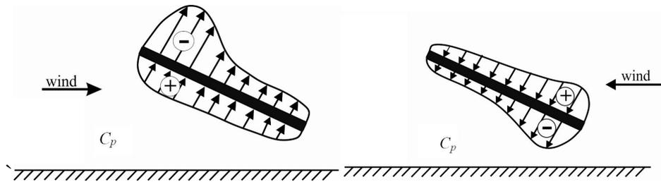
Fig. 3 – Pressure distribution on the surface of the solar panel for north and south wind directions (Ruscheweyh *et al.*, 2011).
