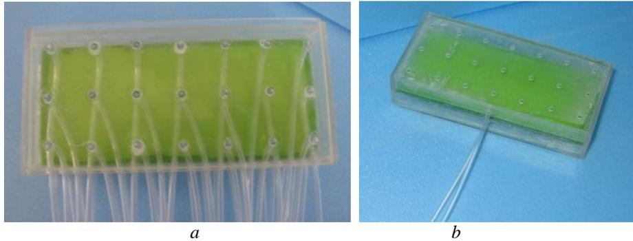
Fig. 5 – The solar panel model: *a* – model used for the local pressure values, *b* – model used for the acquisition of the mean pressure values.
