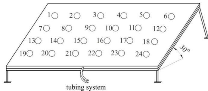
Fig. 2 – The sketch of the solar collector which has been used for the pneumatic pressure averaging method (Radu, Axinte).
