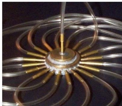
Fig. 1 – Pneumatic manifold proposed by Surry and Stathopoulos (1977).
