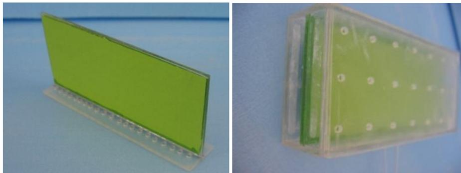
Fig. 4 – Mid-wall as partition inside the models.
