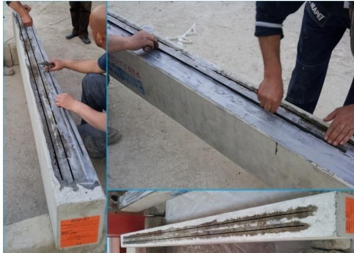
Fig. 3 – Applying of the CFRP strips.
