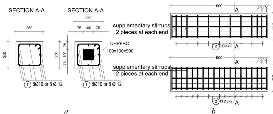
Fig. 5 – Cross section: *a* – transversal; *b* – longitudinal.
