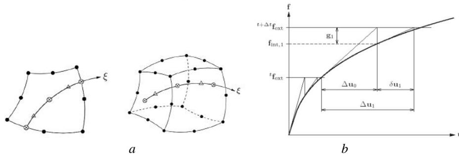
Fig. 1 – Embedded reinforcement in solid (*a*);
