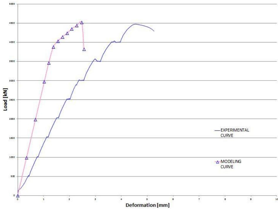
Fig. 6 – Experimental and numerical load – deformation diagram.
