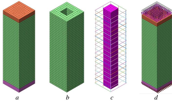
Fig. 3 – *a* – meshed model; *b* – C50/60 mesh; *c* – UHPC core and reinforcement layout; *d* – applied pressure load and supports.
