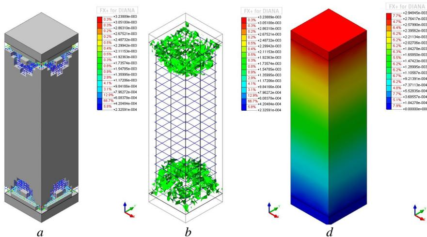
Fig. 4 – *a* – Deformed shape at peak load; *b* – crack model at peak load; *c* – nodal displacement in Z-direction.
