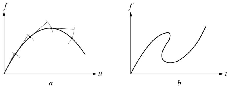
Fig. 2 – *a* – Snap-through behaviour simulated with Arc-Length method;
