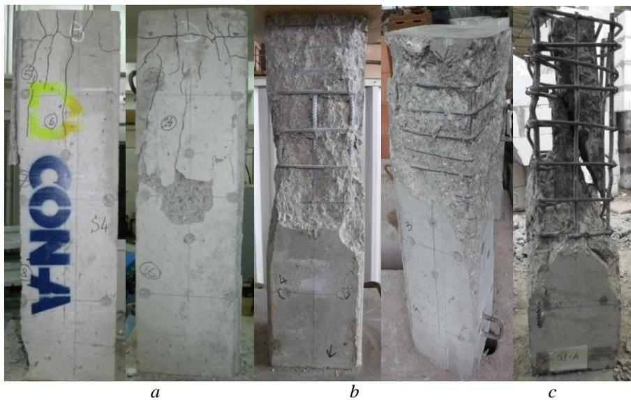
Fig. 7 – Failure modes: *a* – simple columns; *b* – compound columns; *c* – UHPFRC core split.
