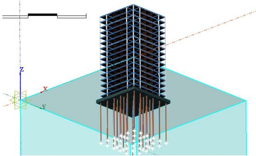
Fig. 2 – Idealized representation of superstructure and foundation system.
