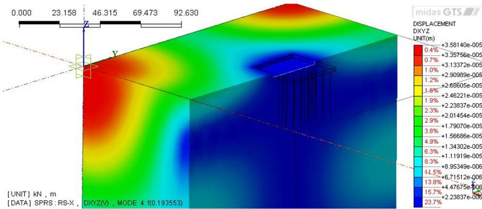
Fig. 6 – The foundation motion in Mode 4 is  $f(0.193 \text{ s})$ .
