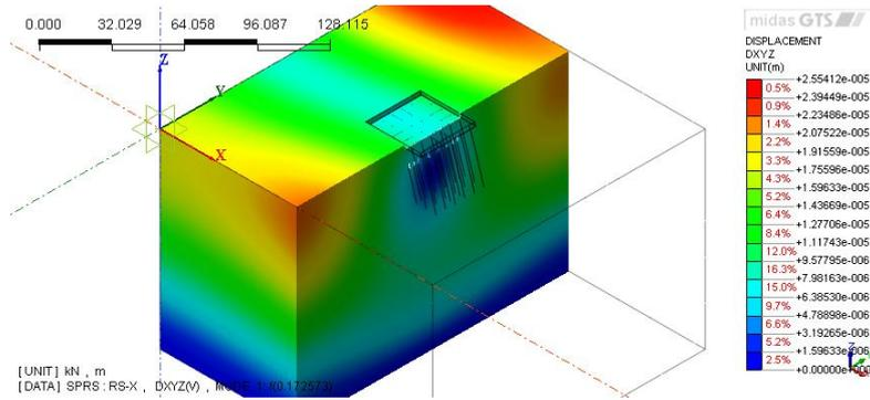
Fig. 16 – The foundation motion in Mode 1 is  $f(0.172\text{ s})$ .
