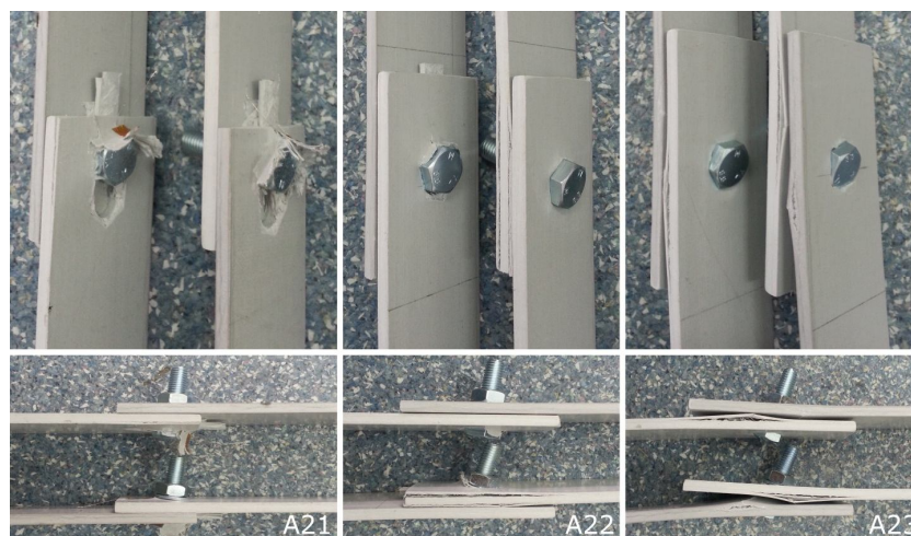
Fig. 5 – Failure modes for bolted joints.
