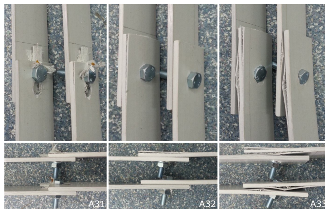
Fig. 7 – Failure modes for bolted joints with bonded inserts.
