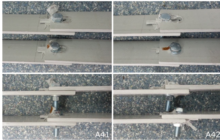
Fig. 9 – Failure modes for bolted joints with tightening torque.
