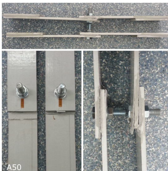
Fig. 11 – Failure modes for hybrid joints (bolted/bonded).
