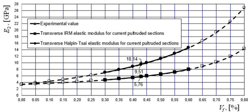
Fig. 4 – The transverse elastic modulus  $E_2$  values obtained using the inverse rule of mixtures (IRM) and Halpin-Tsai equations.
