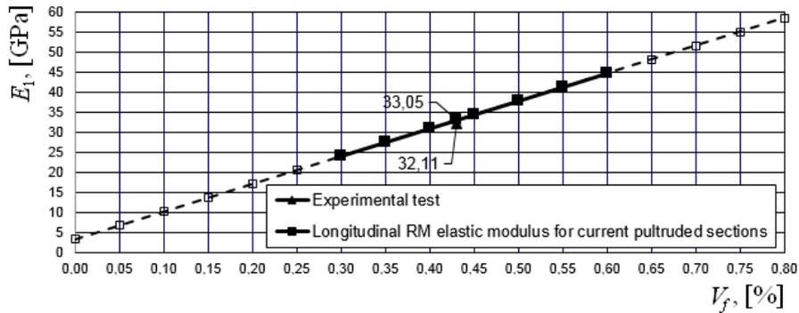
Fig. 2 – The longitudinal elastic modulus,  $E_1$ , values obtained by using the rule of mixtures.
