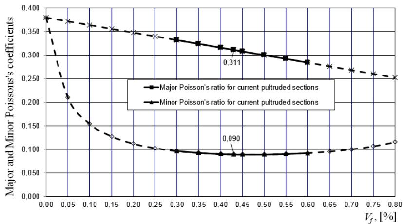
Fig. 6 – Poisson's coefficients in terms of the percentage of the reinforcement,  $V_f$ .
