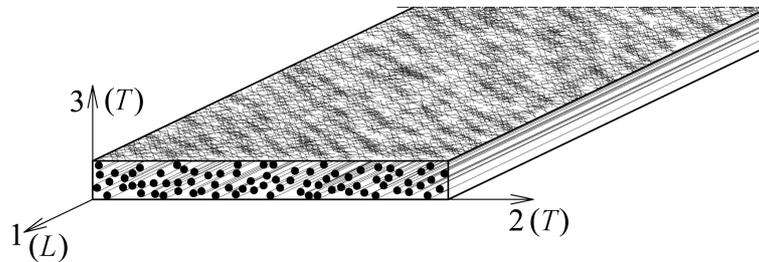
Fig. 1 – The structure of a GFRP pultruded plate.
