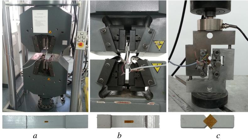
Fig. 3 – Experimental tests on pultruded coupons: *a* – tensile test along the fibres (1); *b* – tensile test normal to the fibres direction (2); *c* – shear test in the plane (1, 2).
