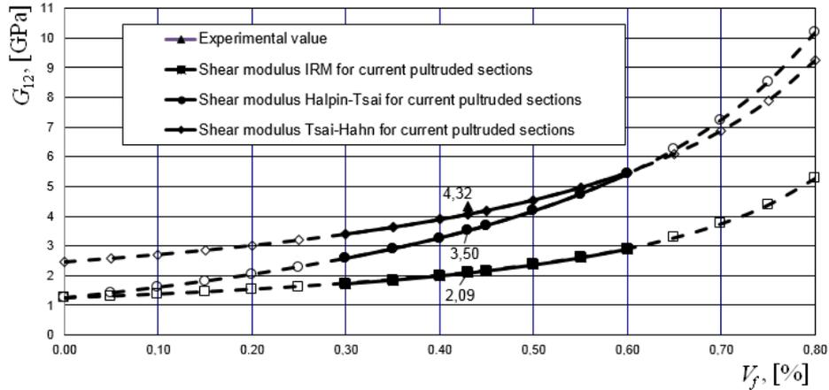
Fig. 5 –The evaluation of the shear modulus  $G_{12}$  using three analytical methods.
