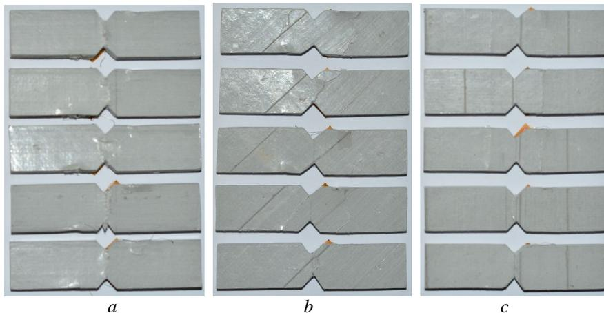
Fig. 4 – Failure modes of the specimens: *a* – longitudinal; *b* – angular; *c* – transverse.
