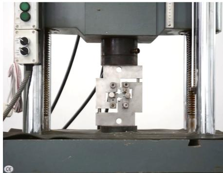
Fig.2 – The universal testing machine and the Iosipescu shear device with the GFRP specimen installed for testing.
