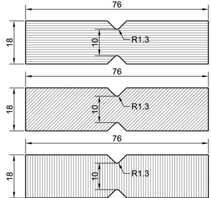
Fig.1 – GFRP specimens with different orientation of fibres: 0°, 45°, 90°.
