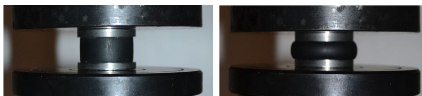
Fig. 2 – The elastomeric specimen fixed without adhesive to metal plates: the undeformed vs. deformed shape.
