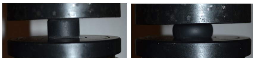
Fig. 3 – The elastomeric specimen fixed without metal plates: the undeformed vs. deformed shape.
