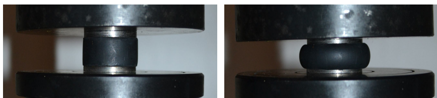
Fig. 1 – The elastomeric specimen bonded to metal plates: the undeformed vs. deformed shape.
